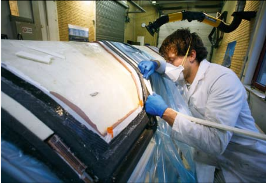
A nine meter long mold serves as the basis of the Superbus' chassis. Layer by layer the carbon fibers are added to create a hard and ultra-rigid frame.
