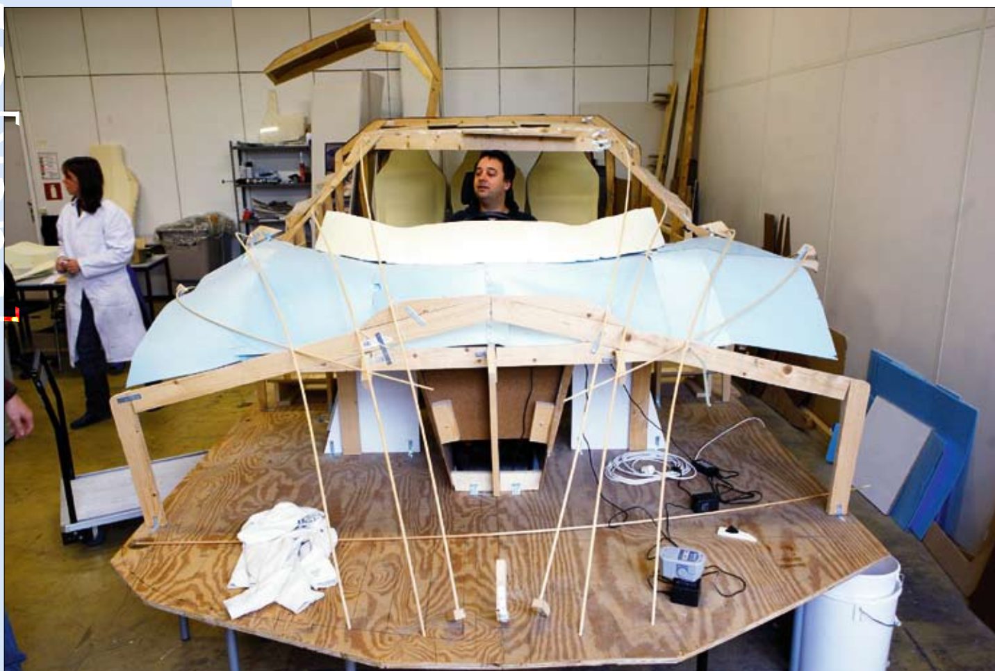
A realistic model is built to optimise the interior, ergonomics and the driver's view.
